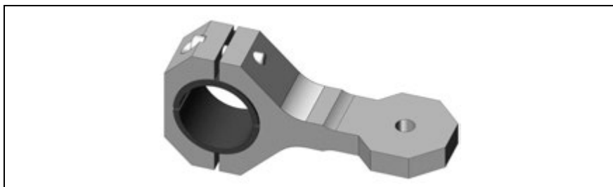
Fig. 3 Mount for the machine cutting torch
