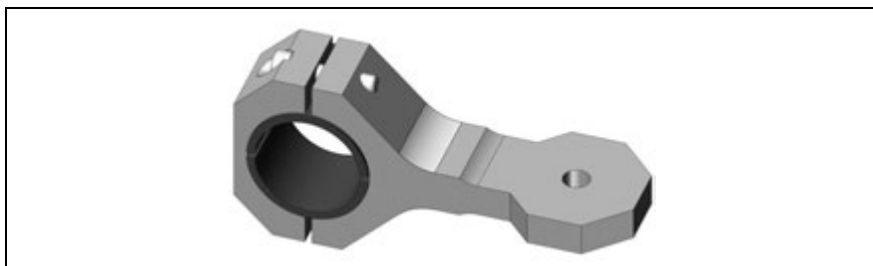
Fig. 3 Mount for the machine cutting torch
